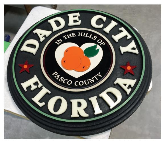
"This sign is a good example of how we use laser-cut acrylic on our work. The HDU panel was cut and carved on the CNC router, then the graphics are all laser cut from different colors of acrylic. I like that the acrylic will look good forever, and I really like how much production time we save."
