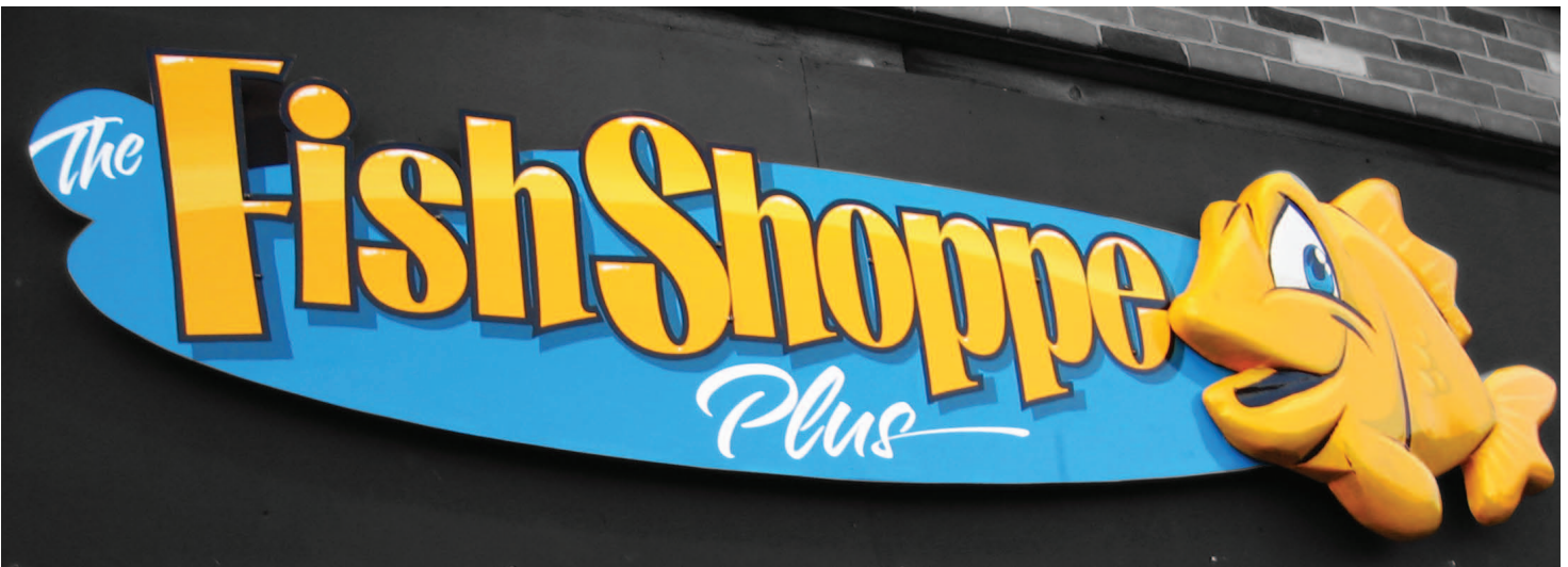
Fish is carved foam coated with Styrospray [www.industrialpolymers.com] on ¼-in. aluminum composite material, finished with 1Shot paints [www.1shot.com]
