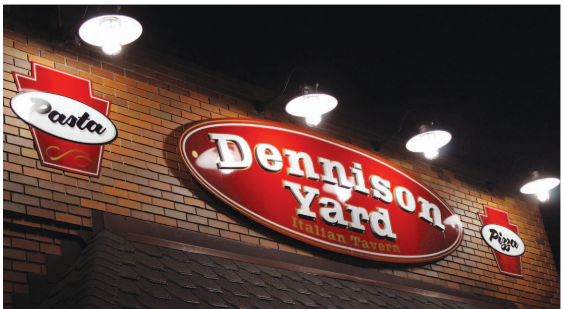
"This is one of the few signs that I didn't design from scratch," says Greg. "This was a redo of their original logo, freshened up a bit. This is ¾-in. overlaid plywood with 3/16-in. aluminum composite material, finished with Ronan paints and Kapco gold metallic vinyl."
