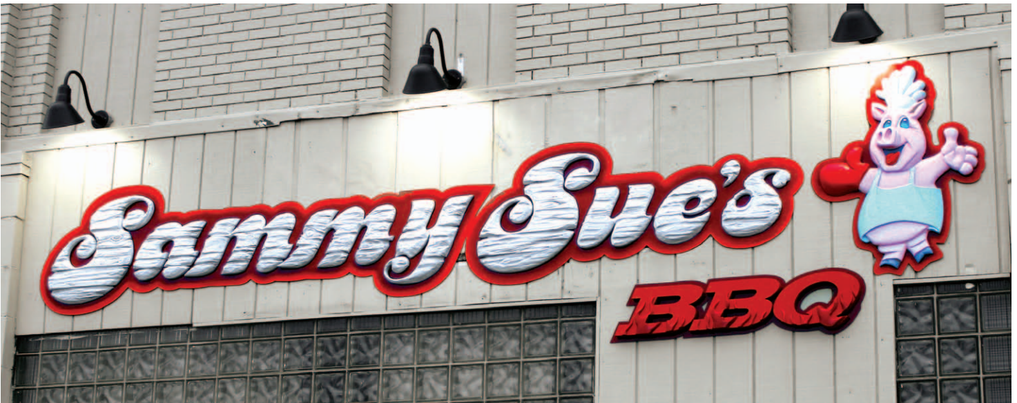
3/16-in. aluminum composite material with 2-in. HDU material. Hand carved woodgrain effect and 3D pig. "This one was a lot of fun," says Greg.
