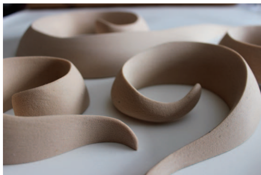
The smoke swirls for the Daily Grind sign were carved from HDU board.
