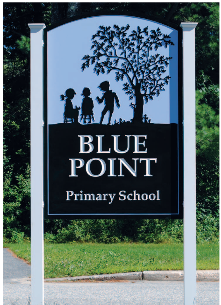
HDU board wrapped with aluminum, on aluminum posts with PVC caps
