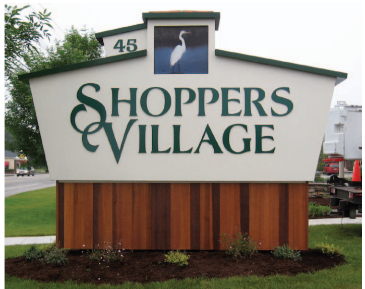
10-by-14-ft. sign with LED-illuminated acrylic letters in aluminum cabinet and copper-topped roof; skirt is cedar.
