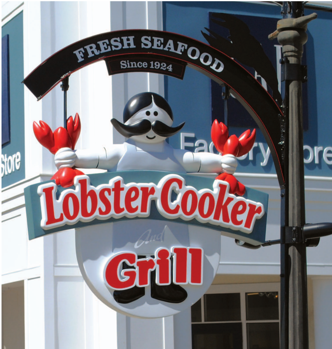
40-by-40-in. HDU board sign on custom aluminum bracket. "This is double-sided," says Bo, "and it's exactly the same on the other side so everything lines up."
