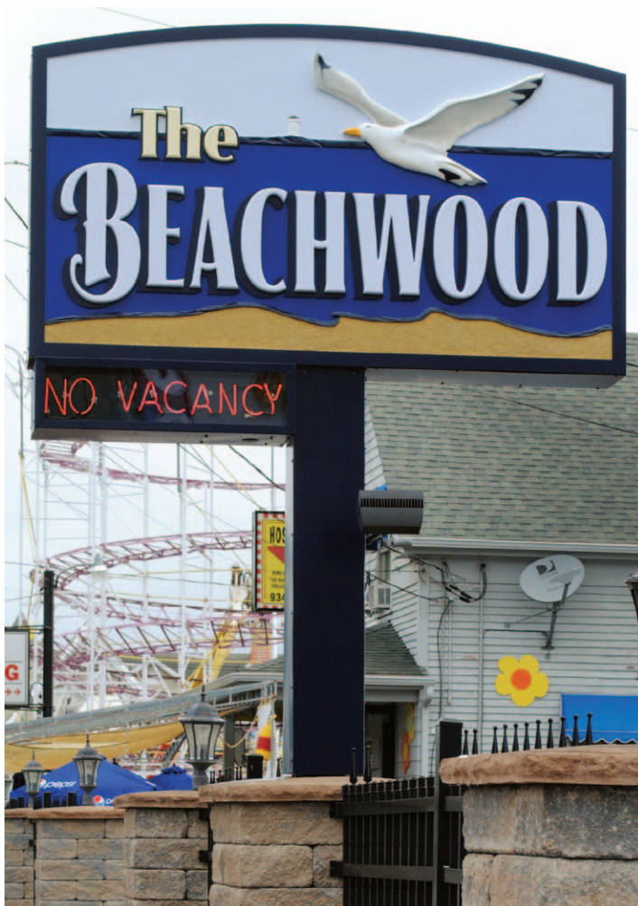
5-by-8-ft. HDU board sign face wrapped with aluminum; beach sand is smalts.
