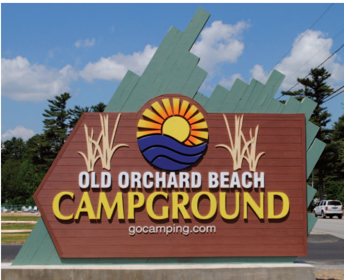
22-by-20-ft. HDU board, aluminum composite and rough sawn timbers
