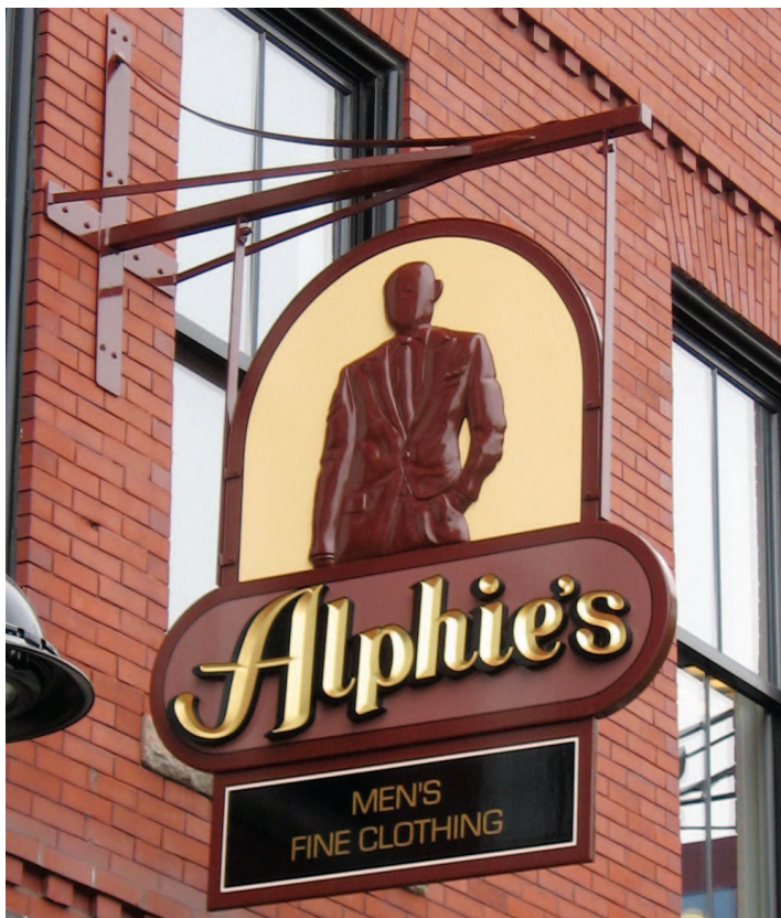
48-by-40-in. carved HDU board, aluminum and overlaid plywood with 23k gold leaf on Alphie's
