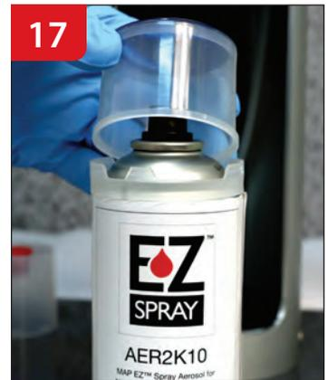
17 Place plastic filling cup with visible color on top of aerosol can.
