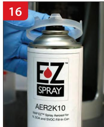
16 Snap plastic adapter ring on top of filled aerosol can.
