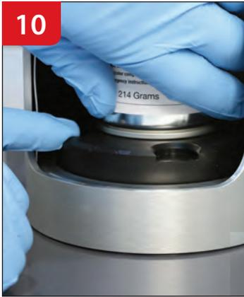
10 Rotate machine's turntable counter-clockwise until aerosol can is seated securely.
