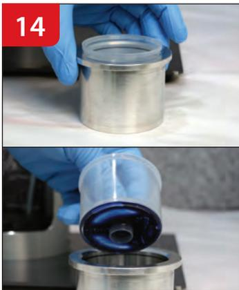
14 On flat non-skid surface, firmly press metal cup downward. This will pop plastic filling cup loose from metal cup.
