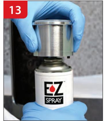
13 Remove metal cylinder cup and plastic filling cup.
