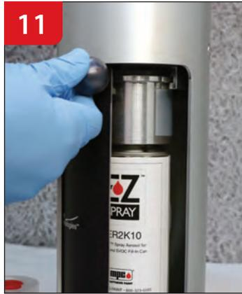
11 Close machine's door to initiate filling (about 3-6 seconds).
