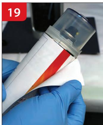
19 Pull black and white label off of aerosol can, revealing the color label.
