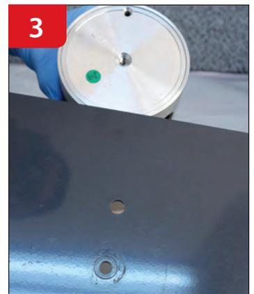
Align the center hole and offset hole in the base plate with the center hole and offset hole in the filling machine.
