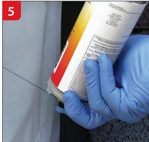
5 Remove top plastic filling cup with color indicator. Facing can away from you, turn can upside down and purge can until a smooth spray pattern is achieved.
