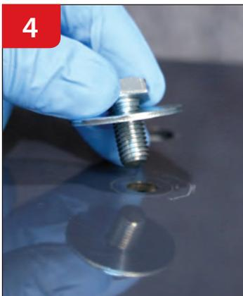
Secure the base plate to the machine with the provided short bolt (not long bolt) and washer through the center holes.
