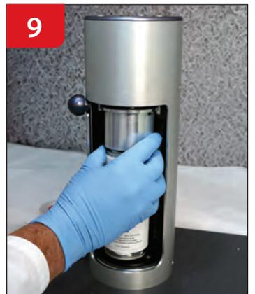
Insert aerosol can with filled
