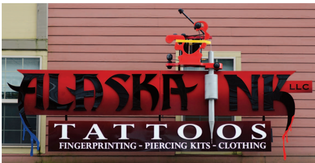
The main sign is 3-by-16-ft., with 35-by-41-in. tattoo gun. "We used a 3mm gloss black Dibond aluminum composite material [ www.graphicdisplayusa.com ] and ¼-in. white acrylic for the lettering," says Jeremy Barry, Sign Pro of Ketchikan, Ketchikan, Alaska. "The fade on the background was done with 1 Shot Bright Red enamel [ www.1shot.com ]. We used 15 lb. Sign Foam HDU [ www.signfoam.com ] for the body and grip of the tattoo gun, and PVC pipe for the machine handle. The gun is finished with 1 Shot enamel, too."
